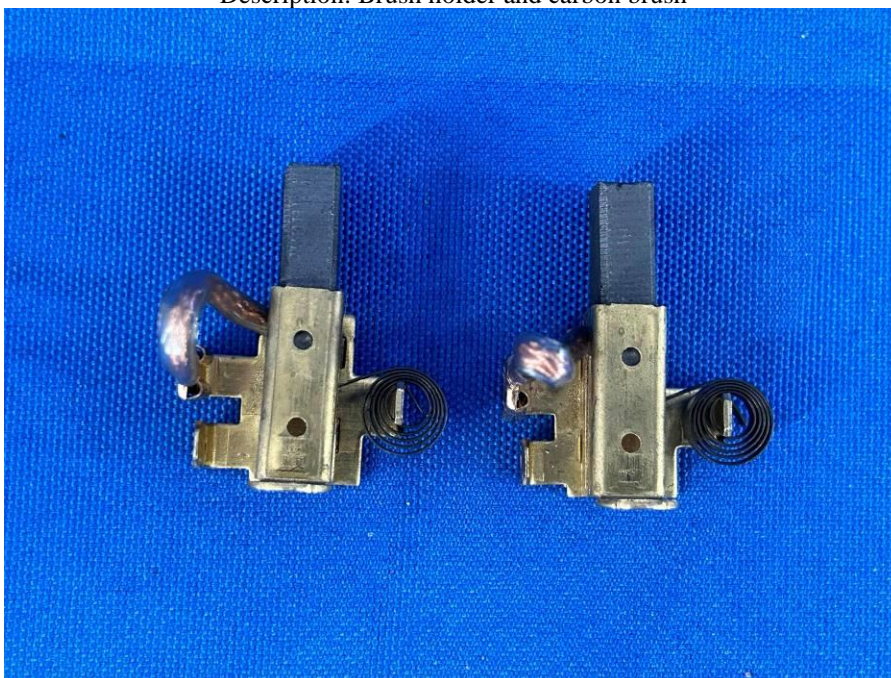
Photo 12 Description: Brush holder and carbon brush
