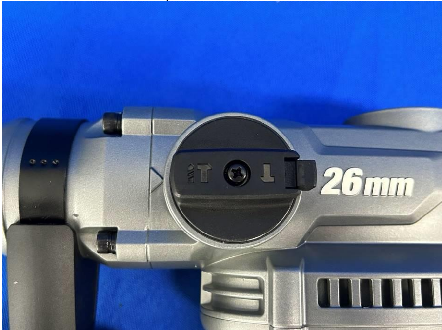
Photo 8 Description: Function control knob
