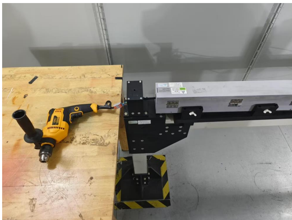
Photograph 2: Set-up for Disturbance Power
