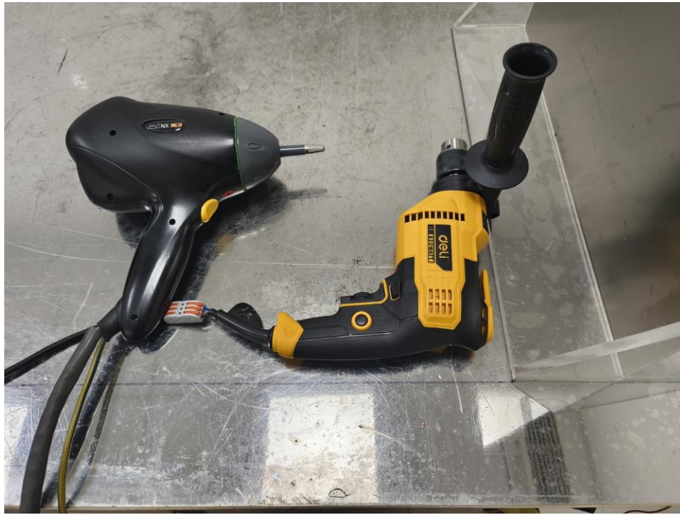
Photograph 3: Set-up for ESD
